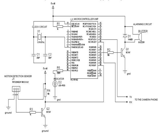
Figure 6: Circuit diagram of the microcontroller connection to PIR sensor.
