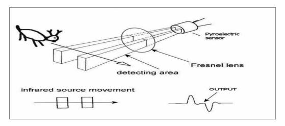
Figure 4: Coverage pattern of the PIR sensor.
