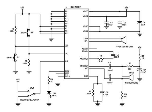
Figure 5: Circuit diagram of the Voice Alert System.
