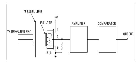
Figure 3: Operational configuration of the PIR sensor.
